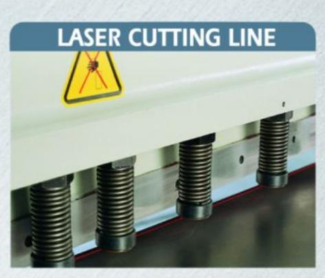
With the help of laser cutting line, angled or drawn line cuttings could be done easily and controllable. (Optional)
