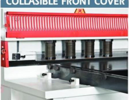
For safety reasons, front side of the hold downs is closed with a protection cover and upon customers' request, 1 m. part on the left side of this cover could be opened. With the help of this system, angled or drawn line cuttings could be done easily and controllable.
