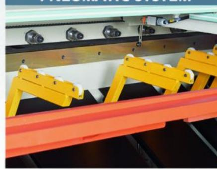
Pneumatic sheet support system that provides the user an easy method of working, is an optional function to protect hanging of sheets down and to improve cutting precision during cutting of long and thin sheets.
