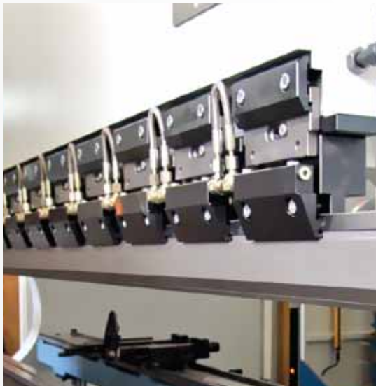
Hydraulic Tool Clamping System (O) Hydraulic tool clamping systems clamp, correct and center the tools, with the help of the hydraulic automatically without need for air. These are perfect solutions to shorten the setup timing and for automated press brakes.
