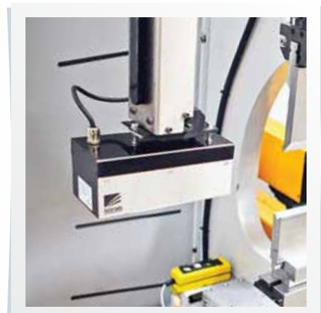
IMG 100 (O) For precision bending, it offers operator safety as well as measuring the bending angle and correction features.
